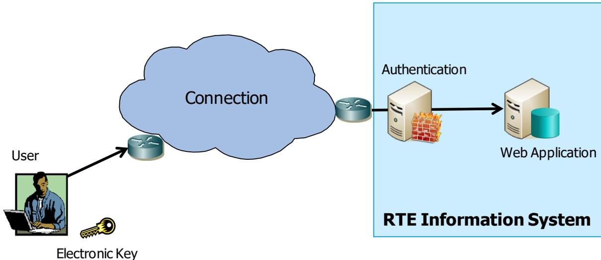
This Method of Use allows any User with access to RTE's IS to log in to the Application from an individual workstation through a browser (pages shown in HTML format).
